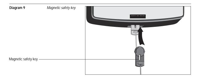
Before you can begin a workout, the magnetic safety key must be inserted into the electronic console as shown in Diagram 9. The treadmill's running belt will not move until the safety key is inserted and secure inside the electronic console.
